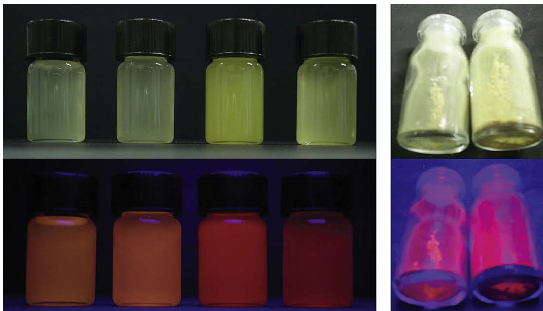
Fig. 8. Quinolones 3a–b under visible light (top) and UV radiation (bottom), where in solution (left): (a) dye 3a in chloroform, (b) dye 3a in dioxane, (c) dye 3b in chloroform and (d) dye 3b in dioxane, and in the solid state (right).
